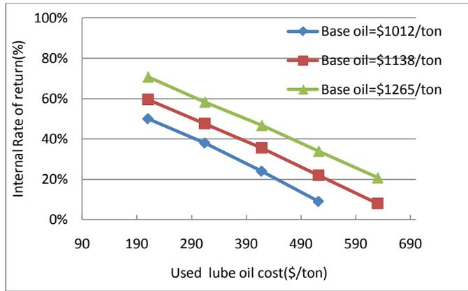
Figure 32 IRR at various feedstock and base oil prices (Base: 40000 metric tons re-refinery)
