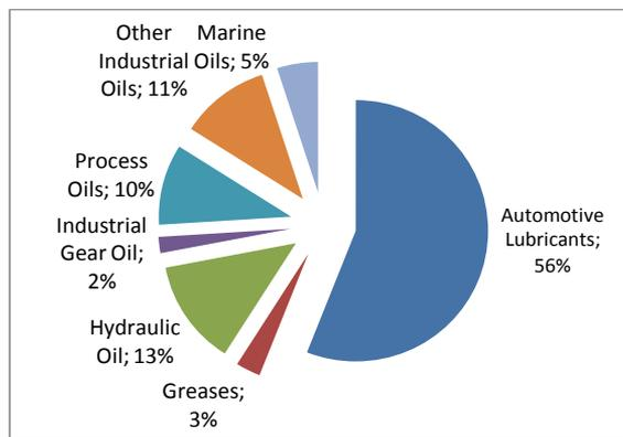
Figure 1 Breakdown of the sources of used lubricating oils
