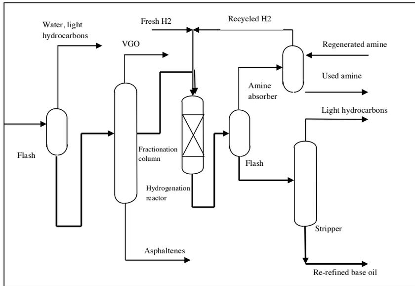
Figure 12 Revivoil simplified process flow diagram
