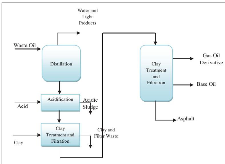
Figure 21 Acid/Clay re-refining process
