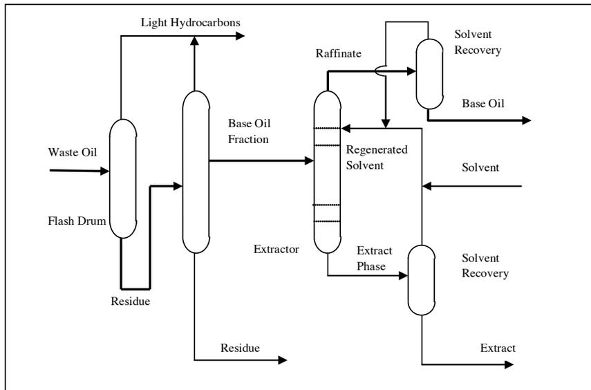
Figure 14 Probex simplified process flow diagram
