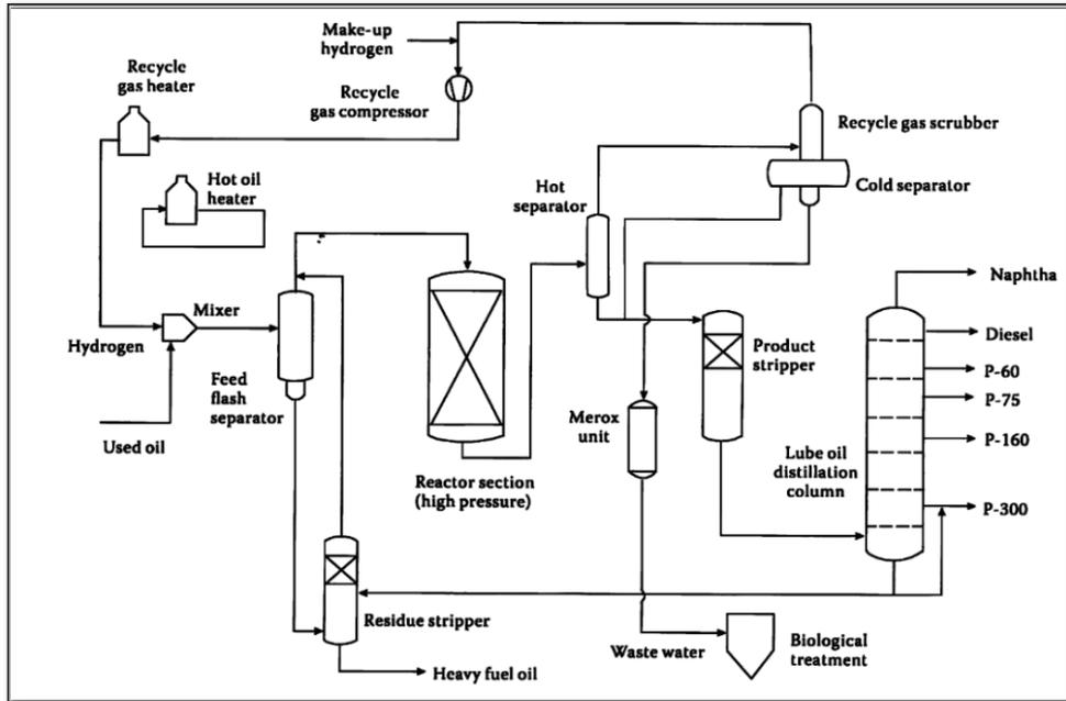
Fig (12) - The Hylube Process - Source 1
