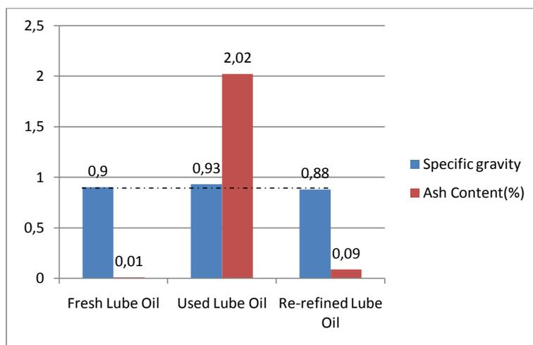
Figure 6 Comparison of Specific Gravity and Ash content before and after re-refining
