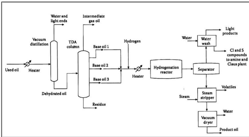
Fig (9) - Simplified Revivoil Process - Source 1
