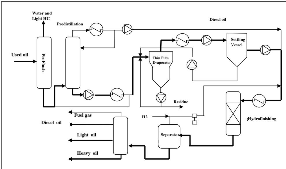
Figure 9 KTI simplified process flow diagram
