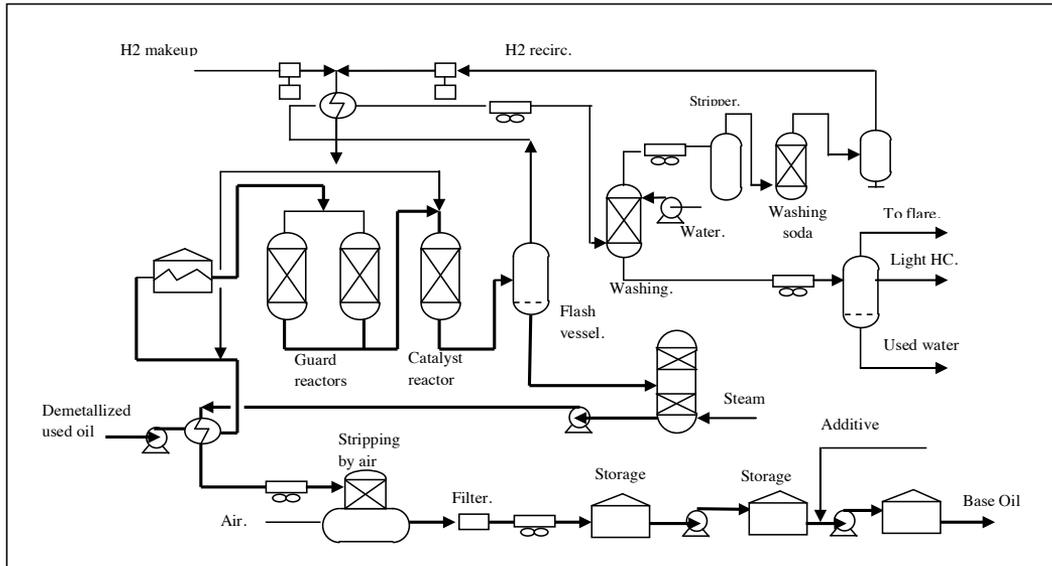
Figure 15 PROP process process flow sheet
