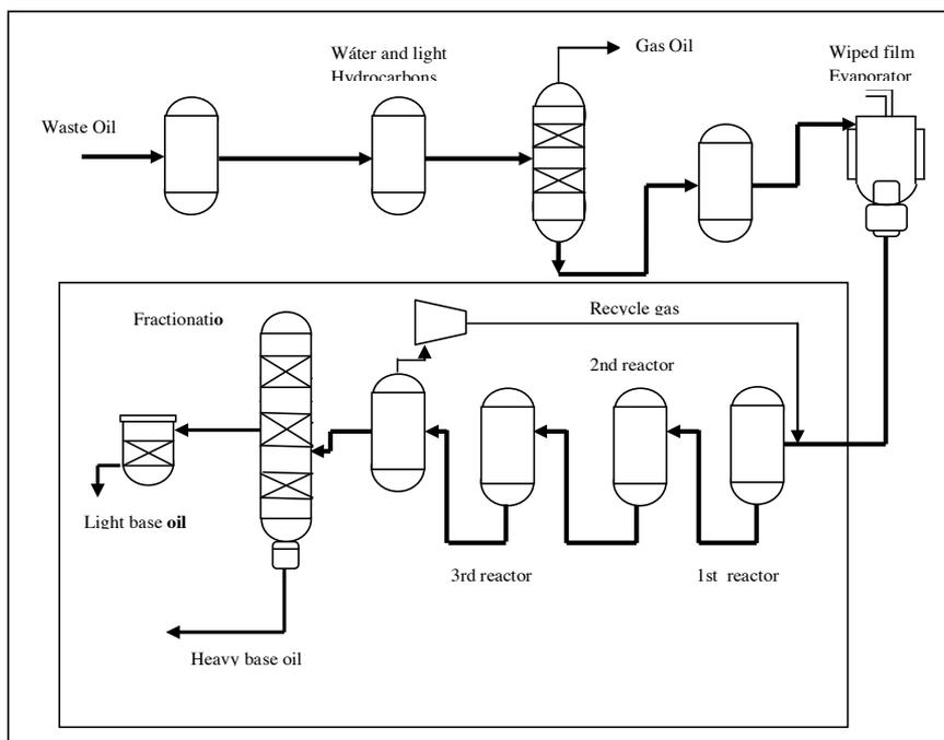
Figure 10 CEP simplified process flow diagram
