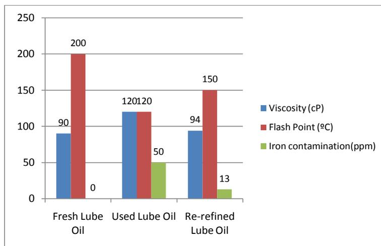
Figure 7 Comparison of Viscosity, Flash Point and Iron content before and after re-refining.
