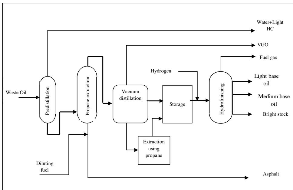
Figure 17 Snamprogetti simplified process flow diagram
