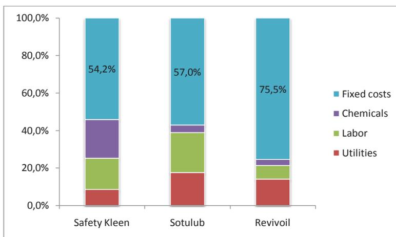
Figure 30 Operating costs for different re-refining technologies
