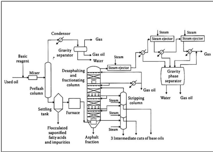
Fig (8) - Original Viscolube Process - Source 1
