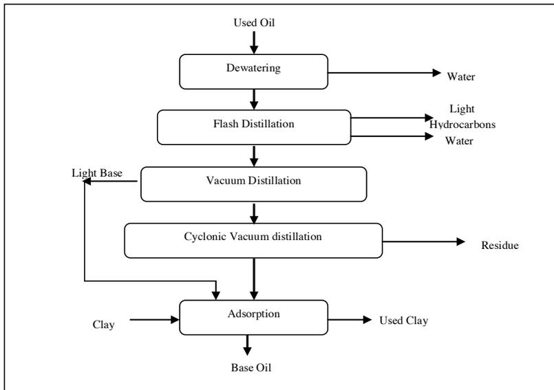
Figure 23 RTI simplified block flow diagram
