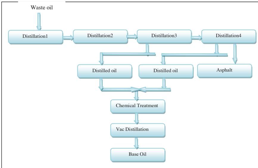
Figure 18 Schematic of the VAXON re-refining process
