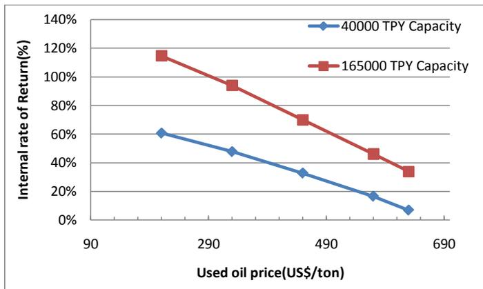
Figure 33 IRR at various feedstock prices and operating capacities at constant base oil price (US\$ 1138 per metric ton)
