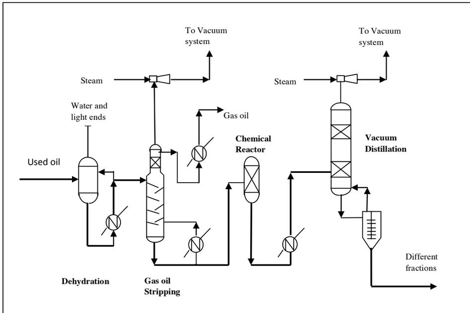
Figure 13 STP simplified process flow diagram
