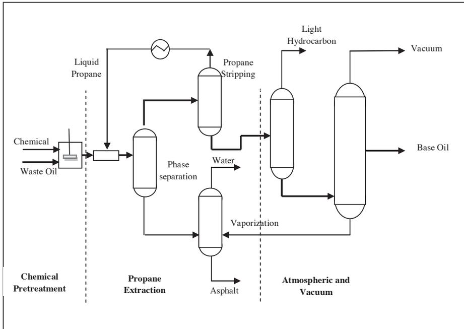
Figure 19 Interline simplified process flow diagram
